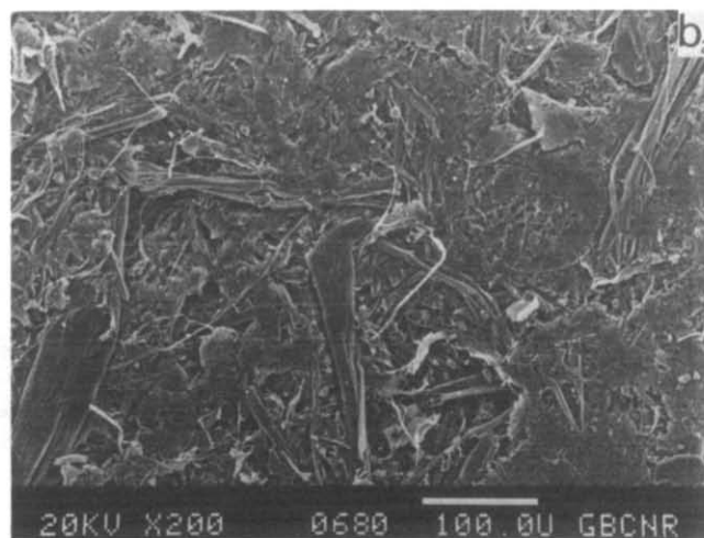
Figure 3 Surface SEM micrograph of plain asbestos (b 1 ) and VP–DVB (14% w/w)–asbestos (b 2 ): untreated samples
